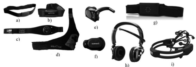
Slika 5: Fiziološki senzori: a) Garmin ANT+ heart monitor, b) Zephyr HxM heart rate monitor c) Zephyr BioHarness 3 physiological monitor, d) Hidalgo Equivital 2 physiological monitor, e) Garmin ANT+ bike and cadence sensor, f) Garmin ANT+ foot pod, g) Zeo sleep monitor, h) NeuroSky MindSet EEG sensor, i) Emotiv EEG neuroheadset
